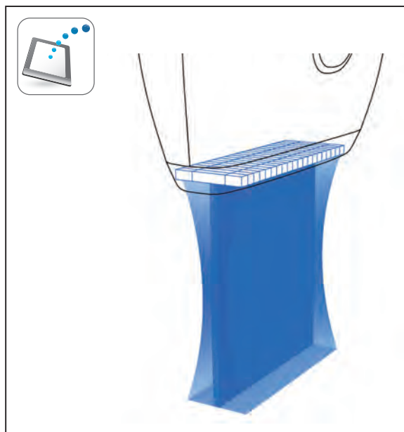
Figure 2. Intelligent Dynamic Micro-Slice (iDMS) technology provides high-flexibility electronic focusing in the lens direction and improves the elevation resolution.
