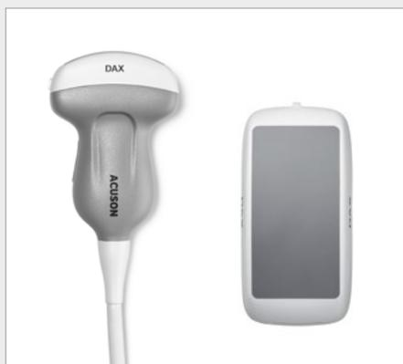
The DAX employs an advanced form of Multi-D beam formation to enable high quality imaging up to 40 cm for the technically difficult patient.
